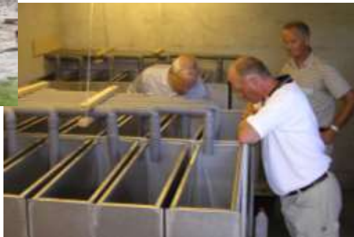
Lysimeter green where drain water can be collected from each experiment plot
